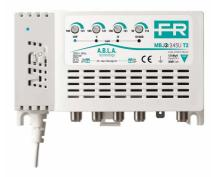
4-input (III+DAB, IV, V, UHF) multiband TV indoor amplifier with 20dB gain and up to 115dBµV output level on UHF band, separate amplification with independent level adjustment (20dB) for each input and low noise figure. Version available with special tuning on the cut between band IV and V and T2 technology with UHF cut band for LTE 4G @790MHz and 5G @694MHz.
